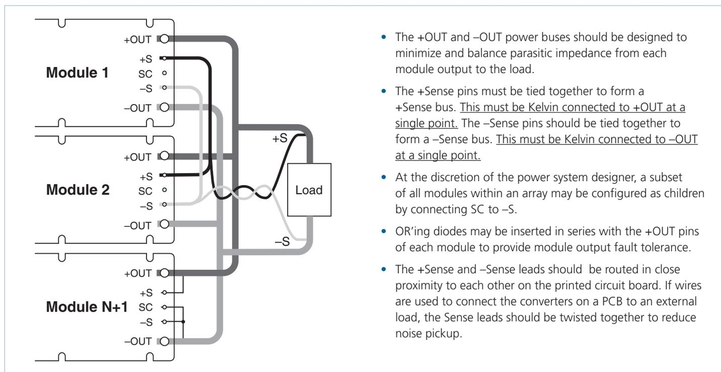
Figure 11 — N+1 module array output connections
