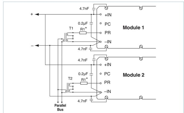
Figure 10 — Transformer-coupled interface
