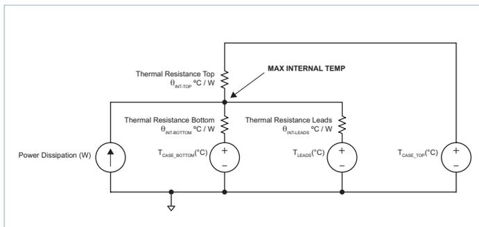
**Figure 23 — Double-side cooling and leads thermal model**
