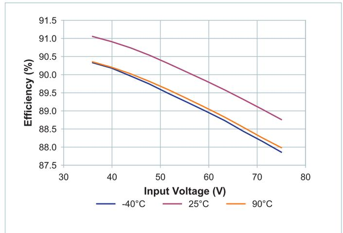
Figure 10 — Full-load efficiency vs.  $V_{IN}$  at nominal trim
