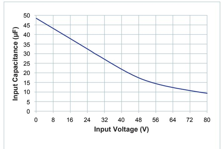
Figure 21 — Effective internal input capacitance vs. applied voltage
