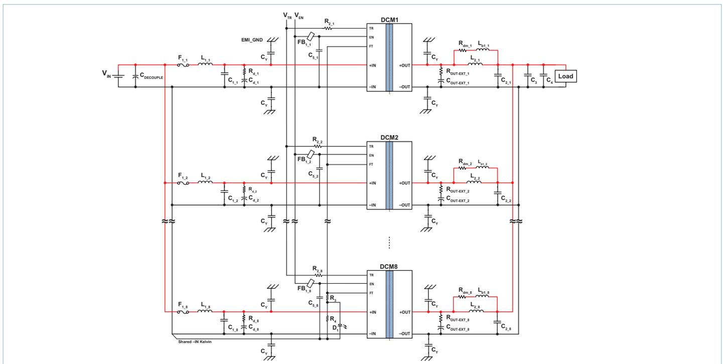
**Figure 26** — DCM paralleling configuration circuit 1
