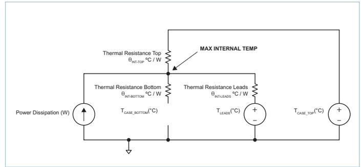
**Figure 24 — One-side cooling and leads thermal model**
